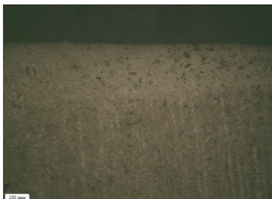
Fig.1. CrB 2 -based layer on D2 die steel.
