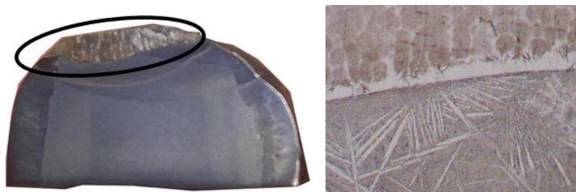
Fig. 1. Main putty, the margin of created white cast iron x100
